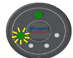
Gas Mode (LED blinking for gas reserve)
