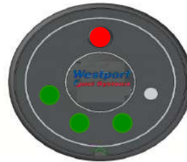
Petrol mode waiting for gas changeover conditions
