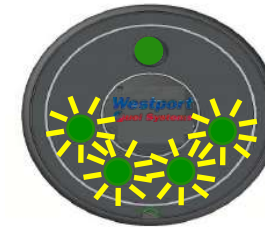
Gas mode refilling over than 80% (4 LEDs blinking green)
