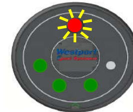
Gas error recording (red LED blinking + Buzzer sound)
